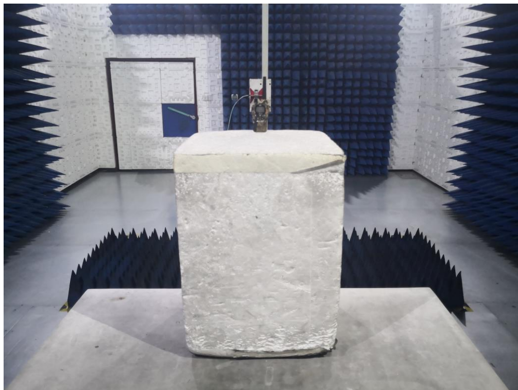
RADIATED EMISSION TEST SETUP ABOVE 1GHz
