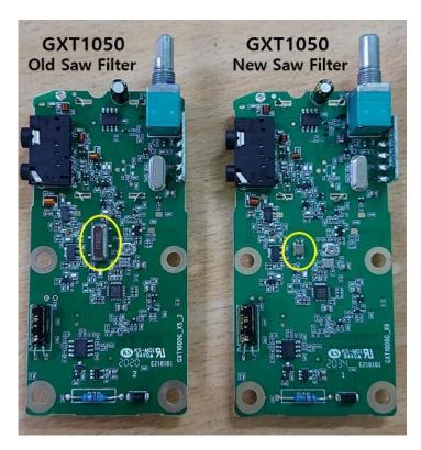
For the above described changes, it does not affect the RF parameters and has no effect on RF Power.We would like to certify the additional of certified FCC ID: MMAGXT1050G as a Class II Permissive Change in this device.
