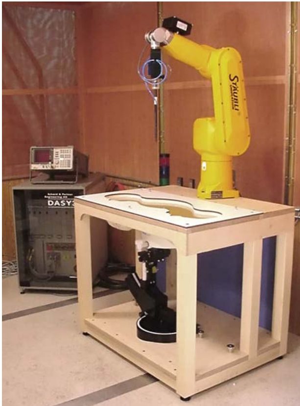
DASY3 SAR Measurement System with SAM Phantom
