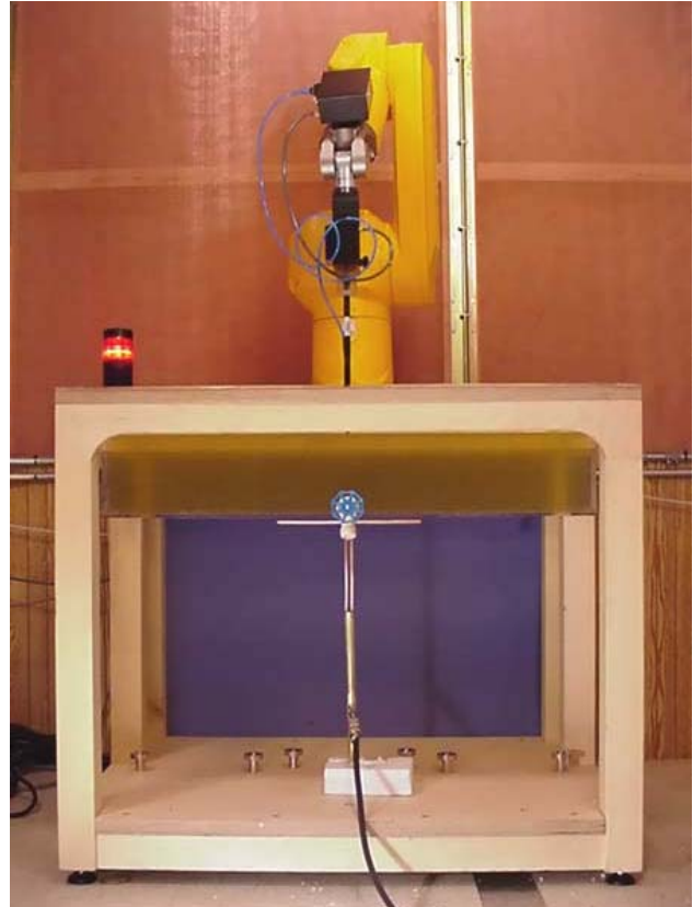
DASY3 SAR Measurement System with validation phantom
