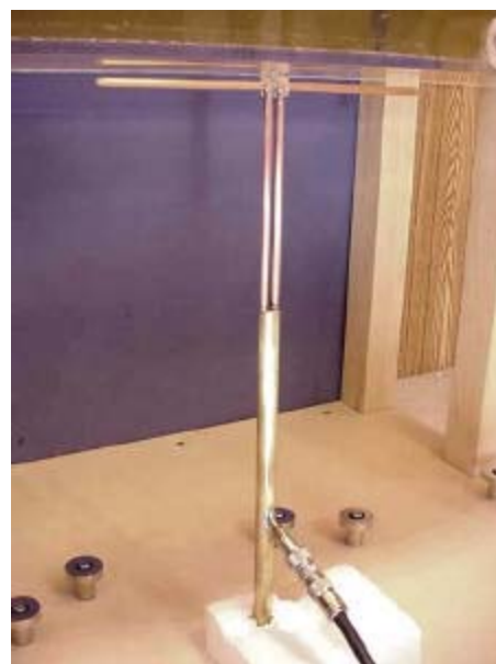
450MHz System Check Setup Photograph
