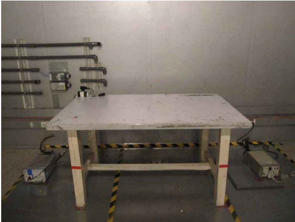
Photograph 2: Set-up for Radiated Emissions, below 1GHz
