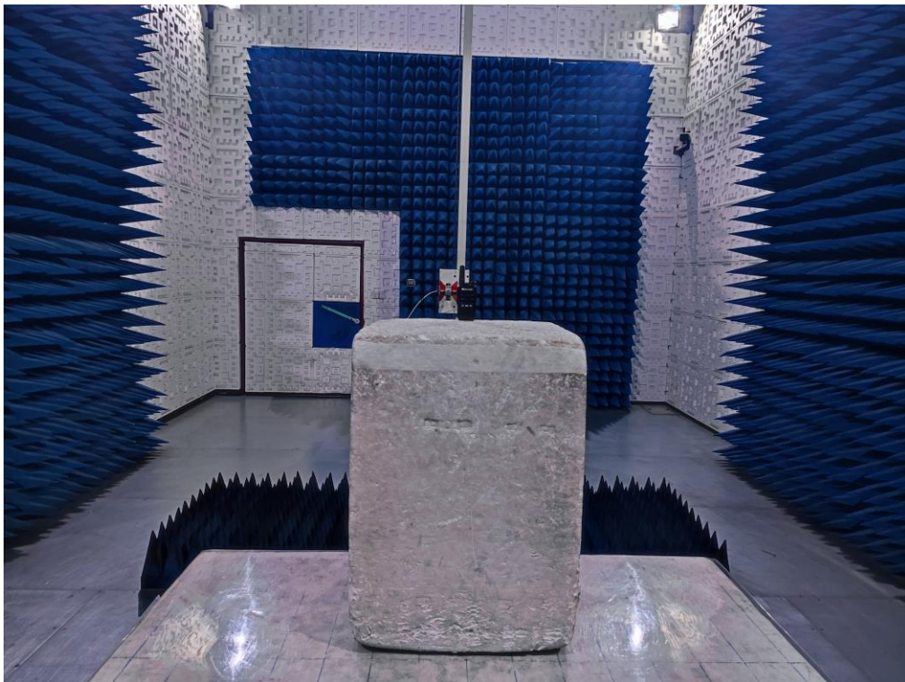
RADIATED EMISSION TEST SETUP ABOVE 1GHz
