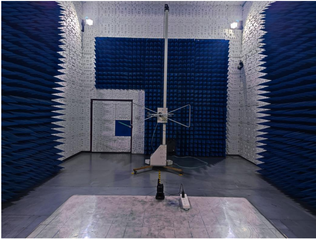
RADIATED EMISSION TEST SETUP ABOVE 1GHz
