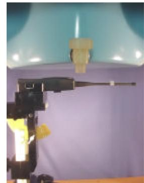
Face-Held SAR Test Setup
