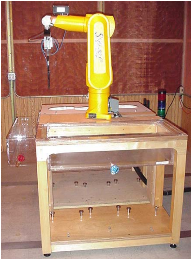
DASY4 SAR Measurement System with validation phantom
