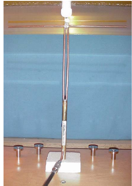
300 MHz Dipole Setup
