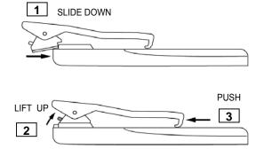
Gently slide the clip into the appropriate guides located in the transceiver's back until it firmly locks.
