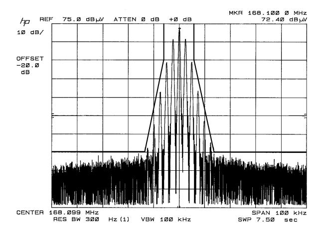
OCCUPIED BANDWIDTH PLOT - 12.5 kHz
