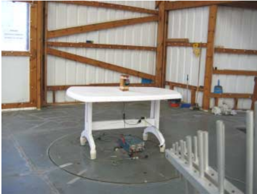
Photograph No.1 Carrier field strength, occupied bandwidth, radiated emissions measurement setup at OATS
