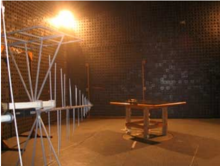
Photograph No.7 Radiated emissions measurement setup in the anechoic chamber with biconilog antenna
