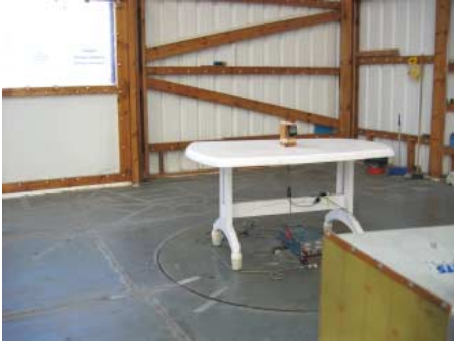
Photograph No.4 Radiated emissions measurement setup at OATS with double-ridged guide antenna
