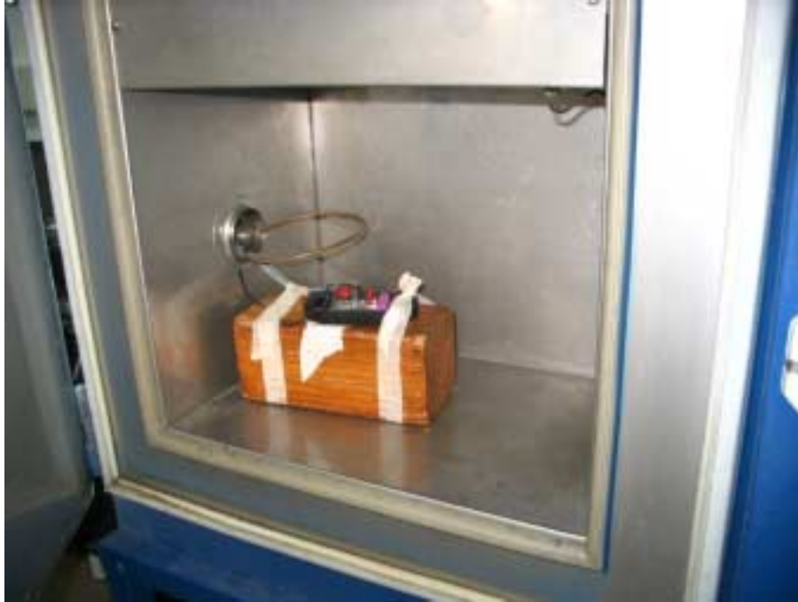
Photograph No.6 Frequency stability measurement setup, EUT close view
