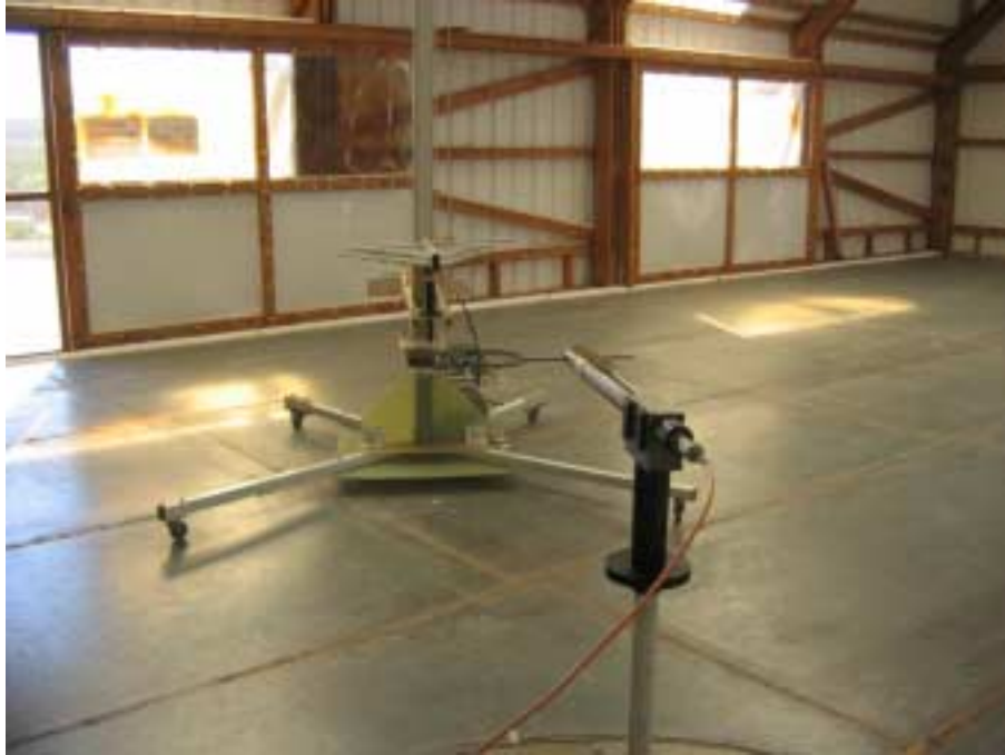
Photograph No.3 Setup for substitution ERP measurements
