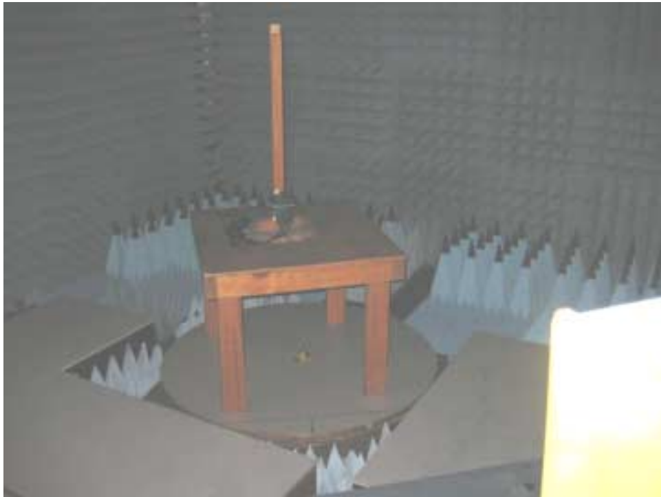
Photograph No.8 Radiated emissions measurement setup in the anechoic chamber with double ridged guide antenna
