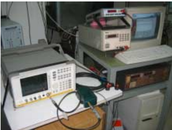
Photograph 7.4.1 Band edge emission measurement set up
