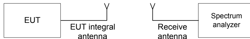
Figure 7.3.1 Emission mask test setup
