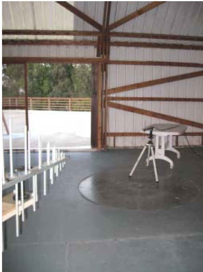
Photograph No.2 Setup for substitution ERP measurements
