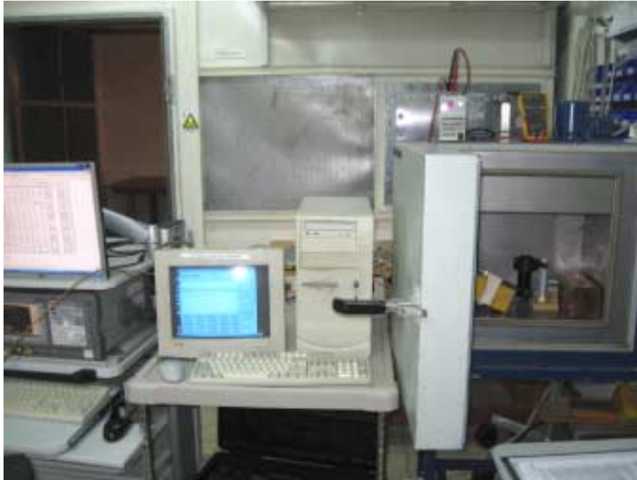
Photograph No.9 Frequency stability measurement setup
