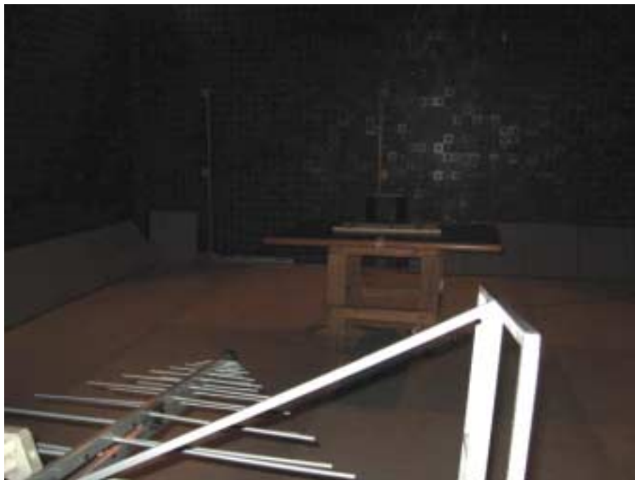
Photograph No.4 Spurious and band edge emissions measurement setup in the anechoic chamber with biconilog antenna
