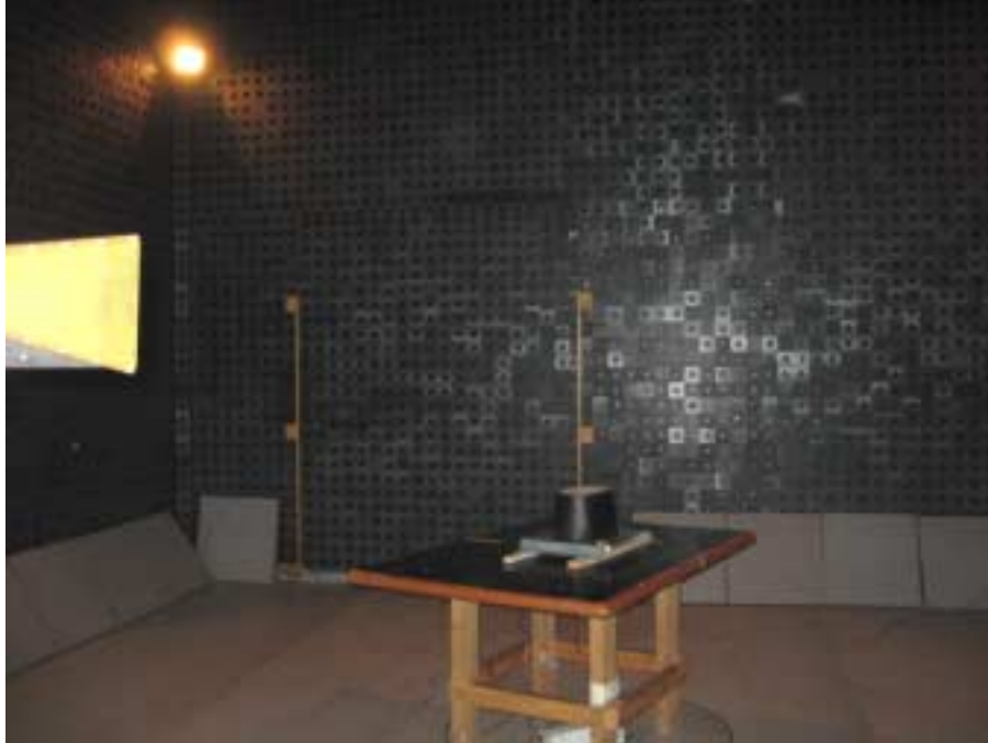
Photograph No.5 Spurious emissions measurement setup in the anechoic chamber with double ridged guide antenna
