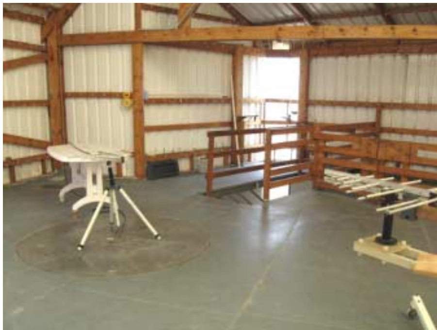
Photograph No.8 Setup for substitution measurements of spurious emissions at the OATS
