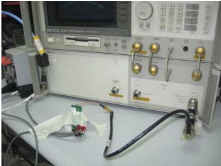
Photograph No.3 Occupied bandwidth test setup
