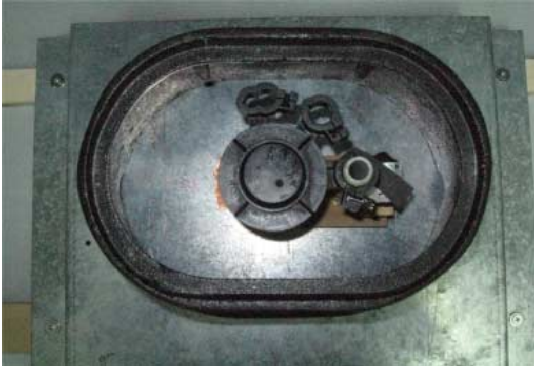
Photograph No.3 Galaxy Pit2 transmitter within metal pit
