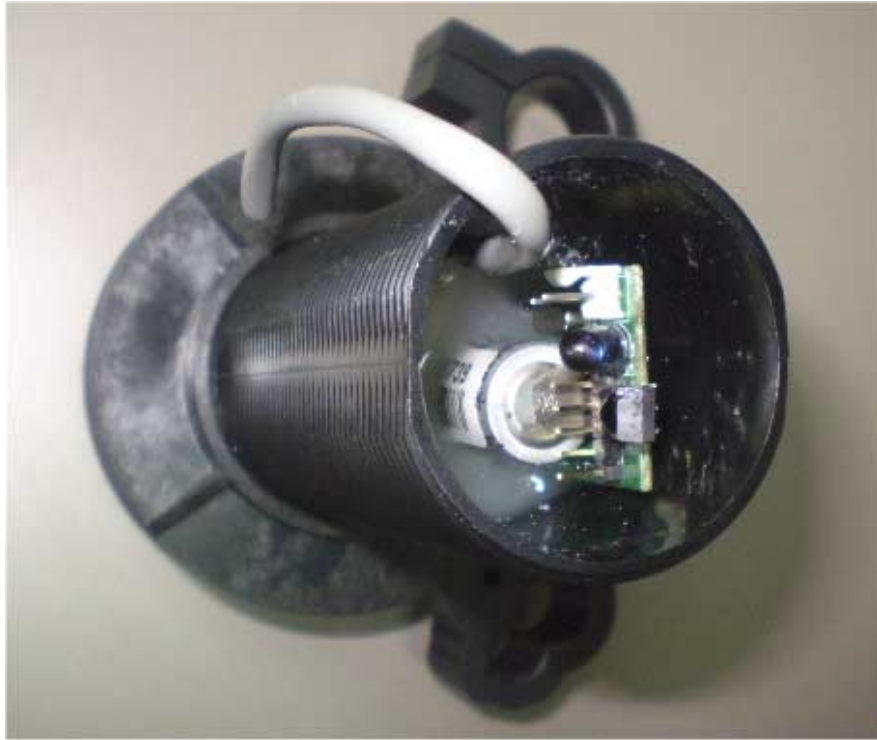
Photograph No.6 Galaxy Pit2 transmitter Bottom view
