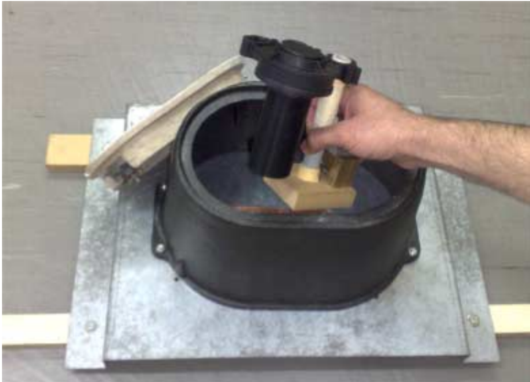
Photograph No.4 Galaxy Pit2 transmitter removed from metal pit
