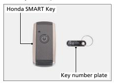
The Honda SMART Key is equipped with a fuel fill cap key and steering lock key.
