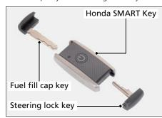
The Honda SMART Key contains electronic circuits that are activated by the Honda SMART Key system. If the circuits are damaged, the Honda SMART Key will not operate.
