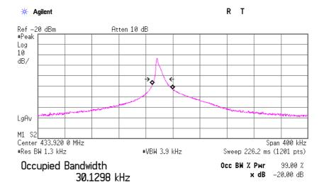
Transmit Freq Error -15.308 kHz x dB Bandwidth 15.601 kHz
