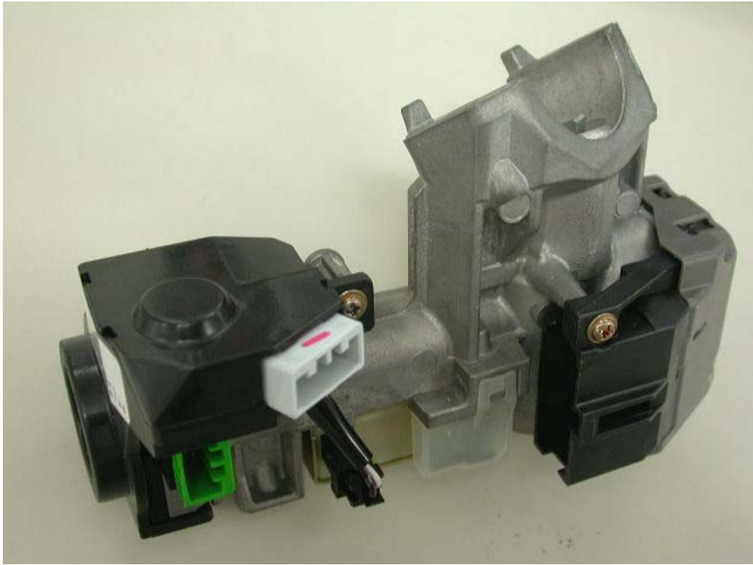
Front of Immobilizer unit and Steering Lock Cylinder
