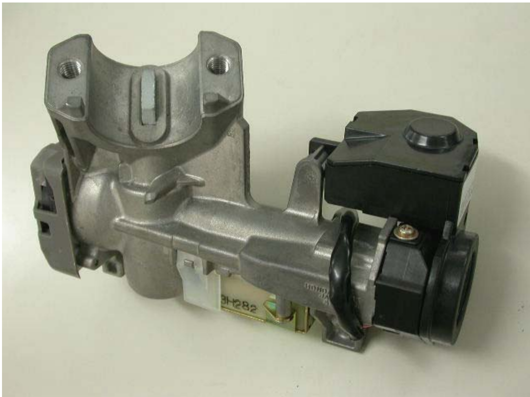
Rear of Immobilizer unit and Steering Lock Cylinder
