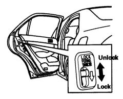
The childproof door locks are designed to prevent children seated in the rear from accidentally opening the rear doors. Each rear door has a lock lever near the edge. With the lever in the LOCK position, the door cannot be opened from inside regardless of the position of the lock tab. To open the door, pull the lock tab up, and use the outside door handle.
