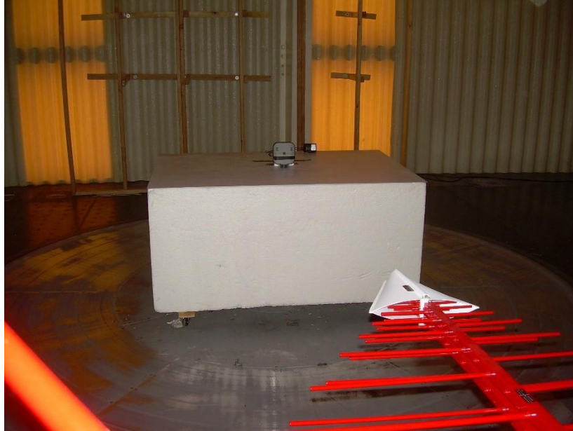
Photograph 1: Front View Radiated Emissions Configuration – 30 – 1000 MHz
