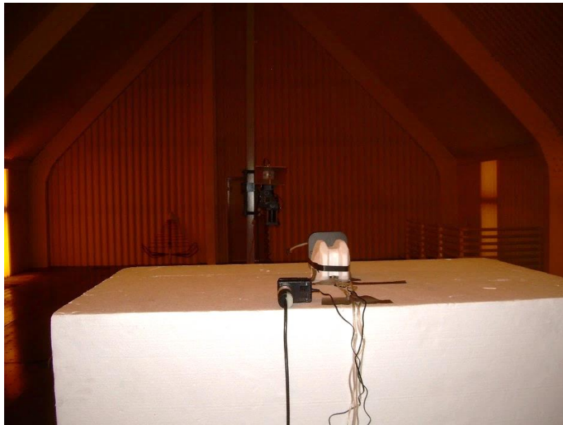
Photograph 4: Back View Radiated Emissions Configuration – Above 1000 MHz
