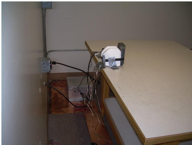
Photograph 6: Back View Conducted Emissions Worst-Case Configuration
