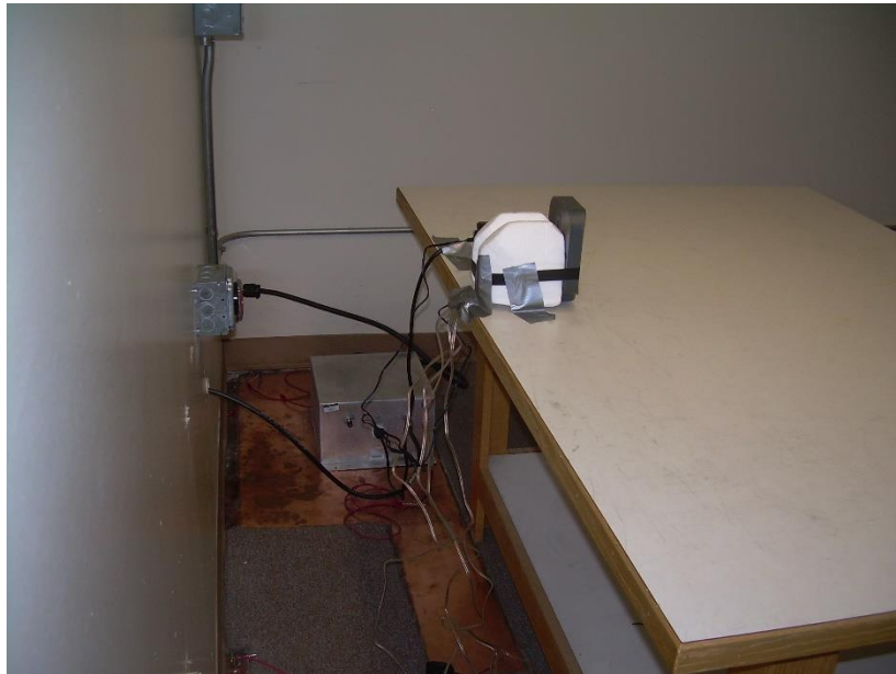
Photograph 6 – Back View Conducted Emissions Worst-Case Configuration
