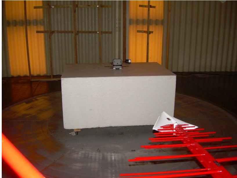
Photograph 1: Front View Radiated Emissions Configuration – 30 – 1000 MHz
