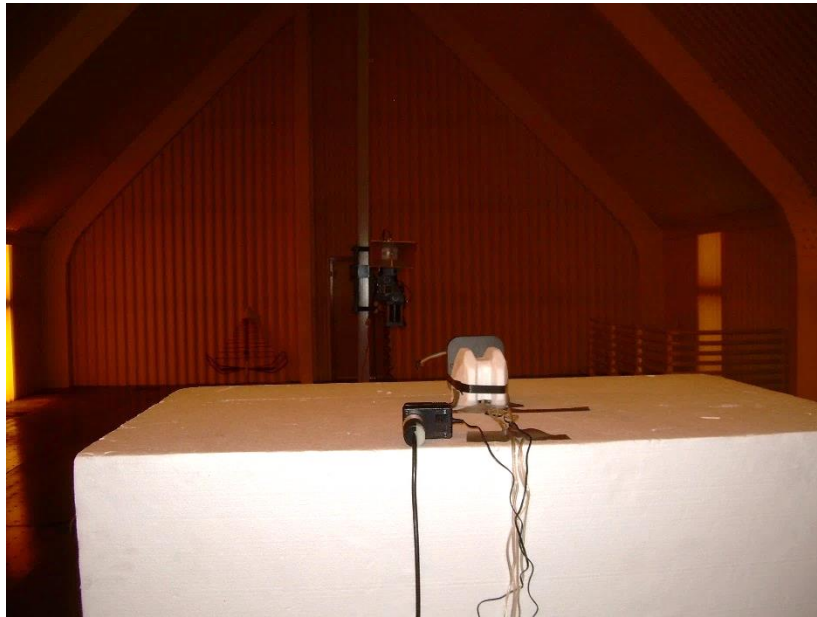
Photograph 4: Back View Radiated Emissions Configuration – Above 1000 MHz
