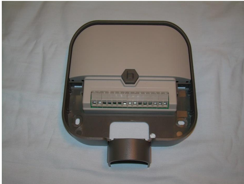
Photograph 12 – Front View of the EUT with Access Panel Removed
