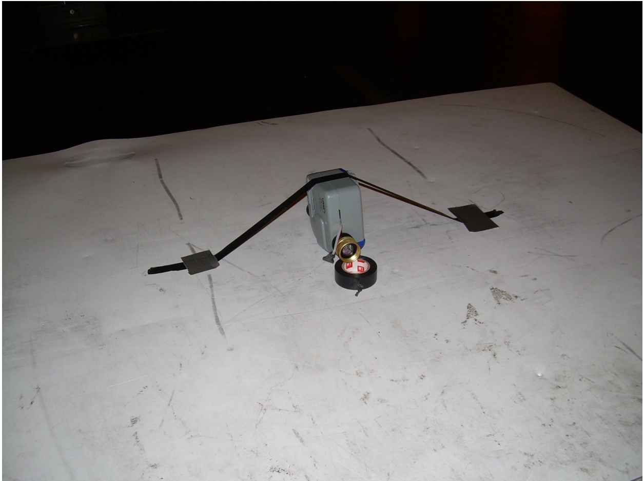
View Radiated Test Setup – On Edge Placement
