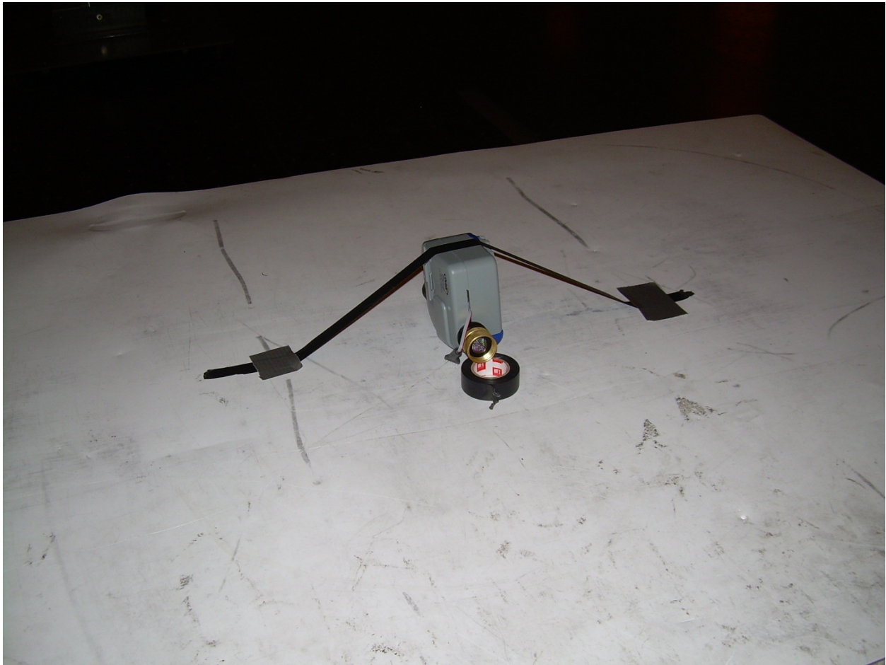
Photograph 2 – View Radiated Test Setup – On Edge Placement
