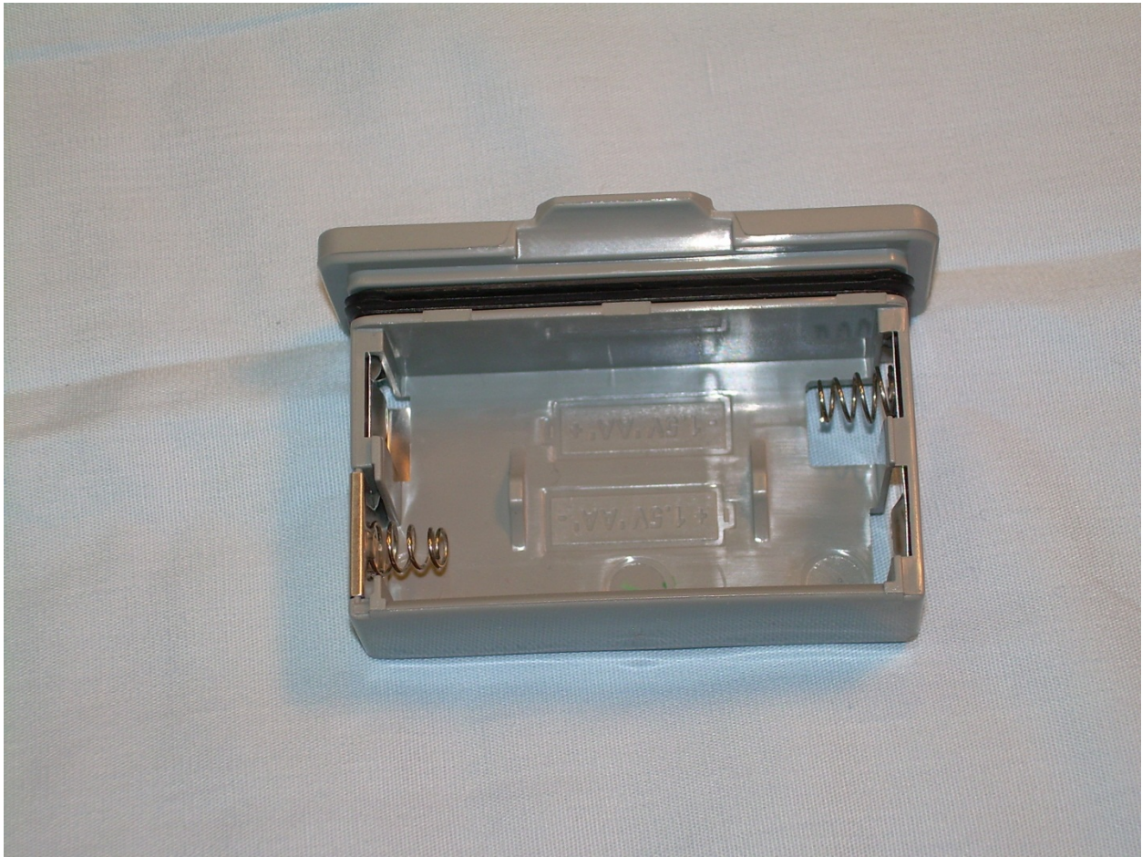
Photograph 7 – View of the Battery Holder – Battery Side
