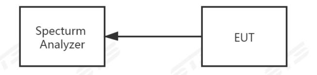
The EUT is connected to the Spectrum Analyzer; the RF load attached to the EUT antenna termina is 50 Ohm; the path loss as the factor is calibrated to correct the reading. Make the measurement with the spectrum analyzer's resolution bandwidth(RBW) = 100 kHz. In order to make an accurate measurement, set the span greater than RBW.
