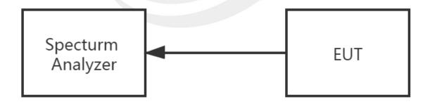
The EUT is connected to the Spectrum Analyzer; the RF load attached to the EUT antenna termina is 50 Ohm; the path loss as the factor is calibrated to correct the reading. Make the measurement with the spectrum analyzer's resolution bandwidth(RBW) = 100 kHz. In order to make an accurate measurement, set the span greater than RBW.
