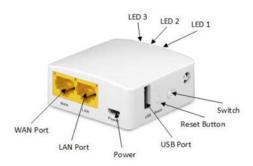
Power to the GLI Mini Router is provided by connect the power lead (supplied) to the power adaptor (buy separately) and then to the power interface on the GLI Mini Router.
