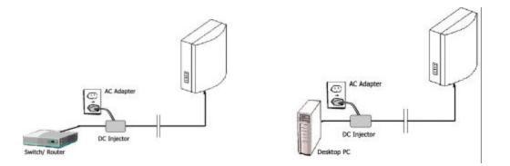
Above: (left) schematic of AVCW-G connected to a network. (right) AVCW-G connected to a terminal PC.
