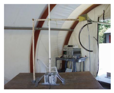
Radiated Emission above 1 GHz Measurement, Omni Antenna, 1-18 GHz, Horizontal
