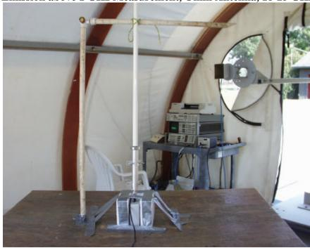
Radiated Emission above 1 GHz Measurement, Omni Antenna, 18-25 GHz, Horizontal
