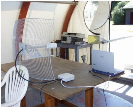
Radiated Emission above 1 GHz Measurement, Parabolic Antenna, 1-18 GHz, Horizontal
