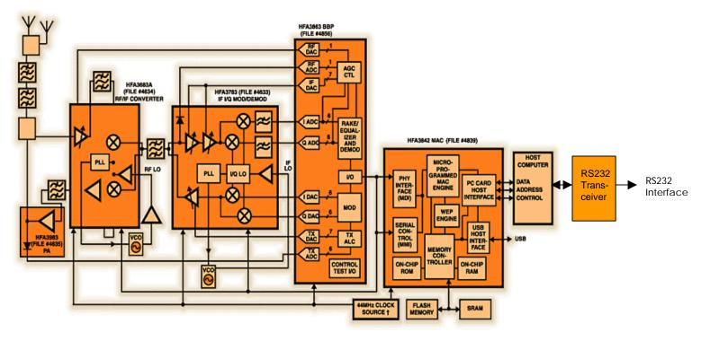
† THE HFA3842 MUST BE SUPPLIED WITH A SEPARATE 48MHz CLOCK WHEN USB IS USED.
