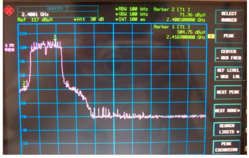
**2**. This is the hard copy of our measurement for EUT communicating with 54Mbps Wireless Lan PC card **channel 13** bandedge.
