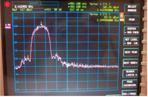
**2**. This is the hard copy of our measurement for EUT communicating with 11Mbps Wireless Lan PC card **channel 11** bandedge.
