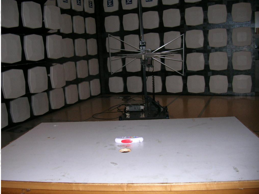
Measurement of Radiated Emission Test Set Up
