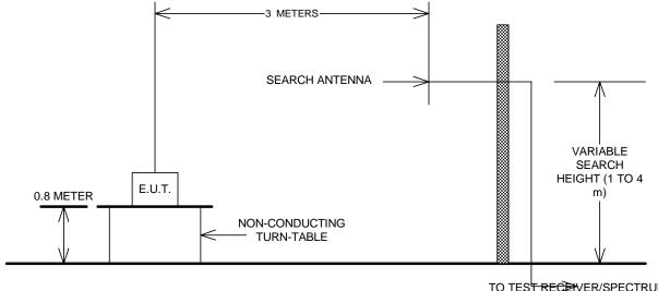
TO TEST RECEIVER/SPECTRUM ANALYZER. A high-pass filter and LNA is necessary to measure to the limits of 15.209.
