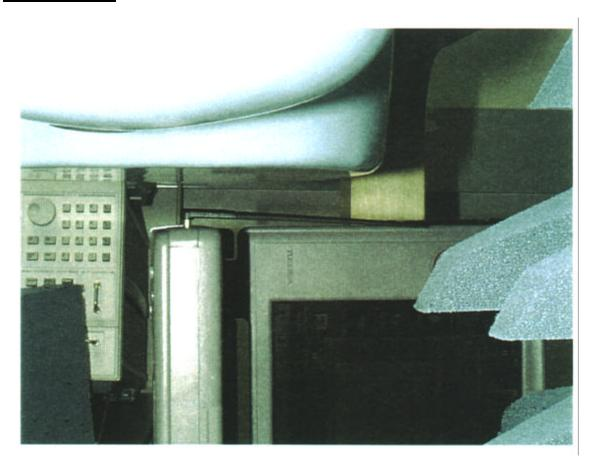
836.01 MHz CDPD Modem, Antenna // Phantom and Pointing Backward, 9/16/98.MEA  $\sigma = 0.95 [mho/m] \quad s_f = 54.0 \quad \rho = 1.00 [g/cm^3]$ Coarse Grid Dx = 15.0 Dy = 15.0 Dz = 0.0 [mm]  $SAR [mW/g] \quad Max: 0.63$ Max at ( 154.50 ,189.00,4.00)
