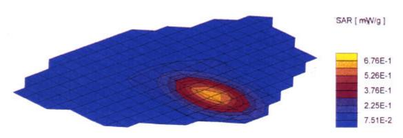
836.01 MHz CDPD Modem, Antenna // phantom and Pointing Forward, 9/16/98.MEA
