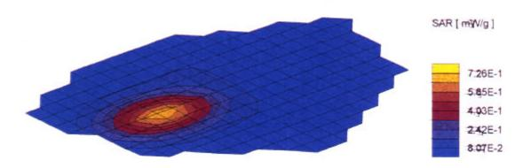
836.01 MHz CDPD Modem, Antenna // Phantom and Pointing Right Side, 9/16/98.MEA  $\sigma = 0.95 \, [\text{mho/m}] \quad \epsilon_f = 54.0 \quad \rho = 1.00 \, [\text{g/cm}^3]$  Cube 5x5x7 Dx = 8.0 Dy = 8.0 Dz = 5.0 [mm]
