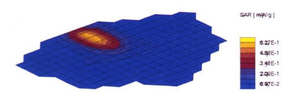
836.01 MHz CDPD Modem, Antenna // Phantom and Pointing Backward, 9/16/98.MEA  $\sigma = 0.95 \frac{[mho/m]}{[mho/m]} = 54.0 \quad \rho = 1.00 \frac{[g/cm^3]}{[mm]}$   $Cube 5x5x7 \quad Dx = 8.0 \quad Dy = 8.0 \quad Dz = 5.0 \quad [mm]$   $SAR [mW/g] \quad Max: 0.89$   $SAR (fg): \quad 0.618 \quad [mW/g] \quad SAR (f0g): \quad 0.437 \quad [mW/g]$
