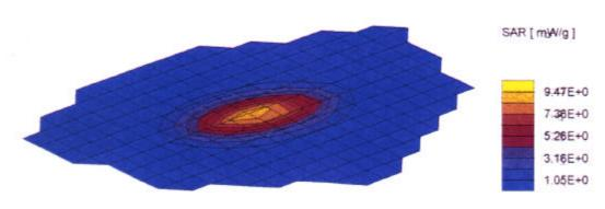
900 MHz Verification 9/16/98.MEA  $_{0}$  = 0.87 [mho/m]  $_{E_{f}}$  = 41.4  $_{p}$  = 1.00 [g/cm<sup>3</sup>] Cube 5x5x7 Dx = 8.0 Dy = 8.0 Dz = 5.0 [mm] SAR [ mW/g ] Max: 14.24 SAR (1g): 9.04 [mW/g] SAR (10g): 5.89 [mW/g]
