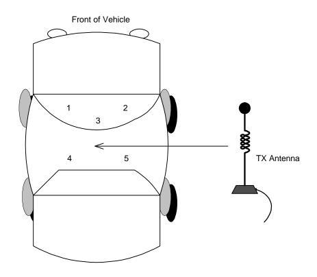
Test #4 - Measurements Inside Vehicle With Antenna Mounted At Rear
