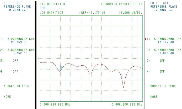
Return loss with 4.4mm separator
