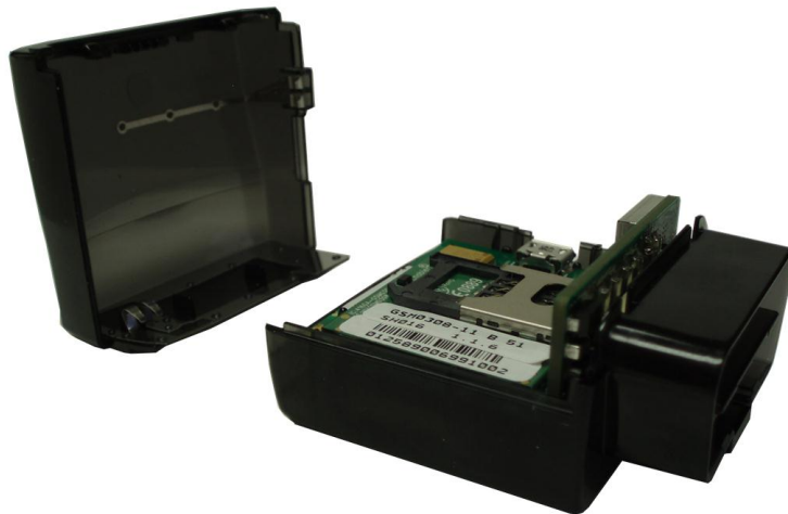
Figure: 10 - MT 3050 With Cover Removed
