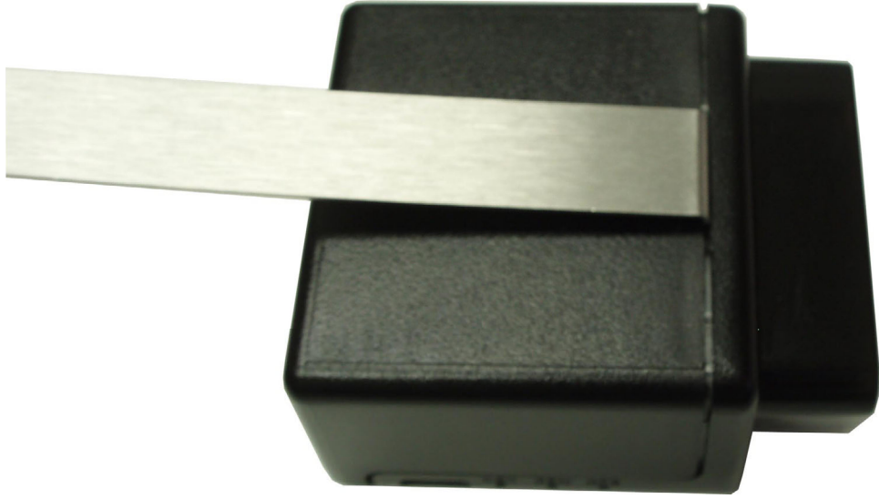
Figure: 8 - Lever inserted into MT 3000 lid gap
