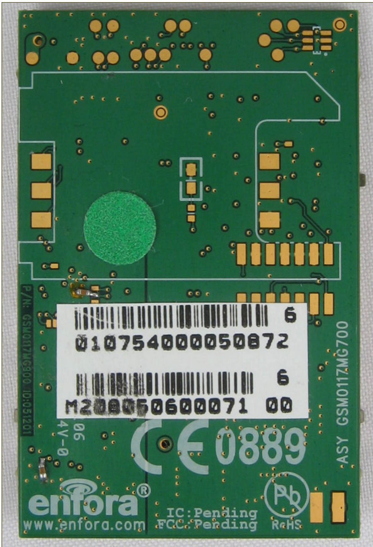
Figure 5: Solder side of board with cardholder removed
