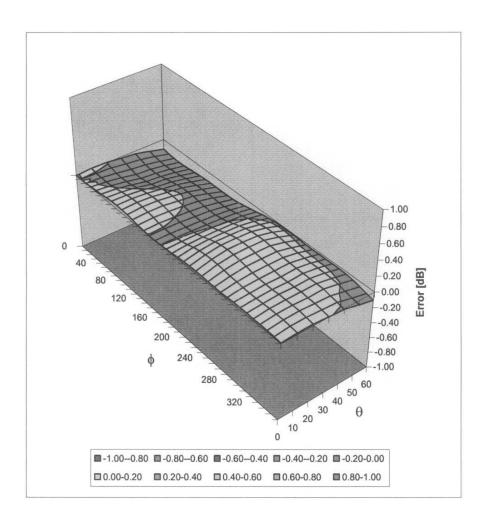
Spherical Isotropy Error < ± 0.4 dB
