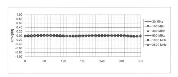
Axial Isotropy Error < ± 0.2 dB
