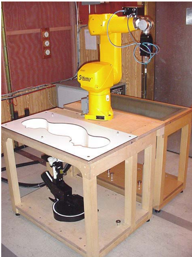
DASY4 SAR Measurement System with SAM Phantom
