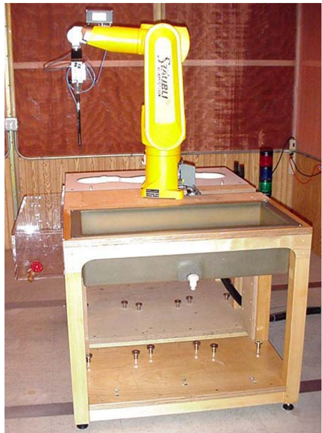
DASY4 SAR Measurement System with Planar Phantom
