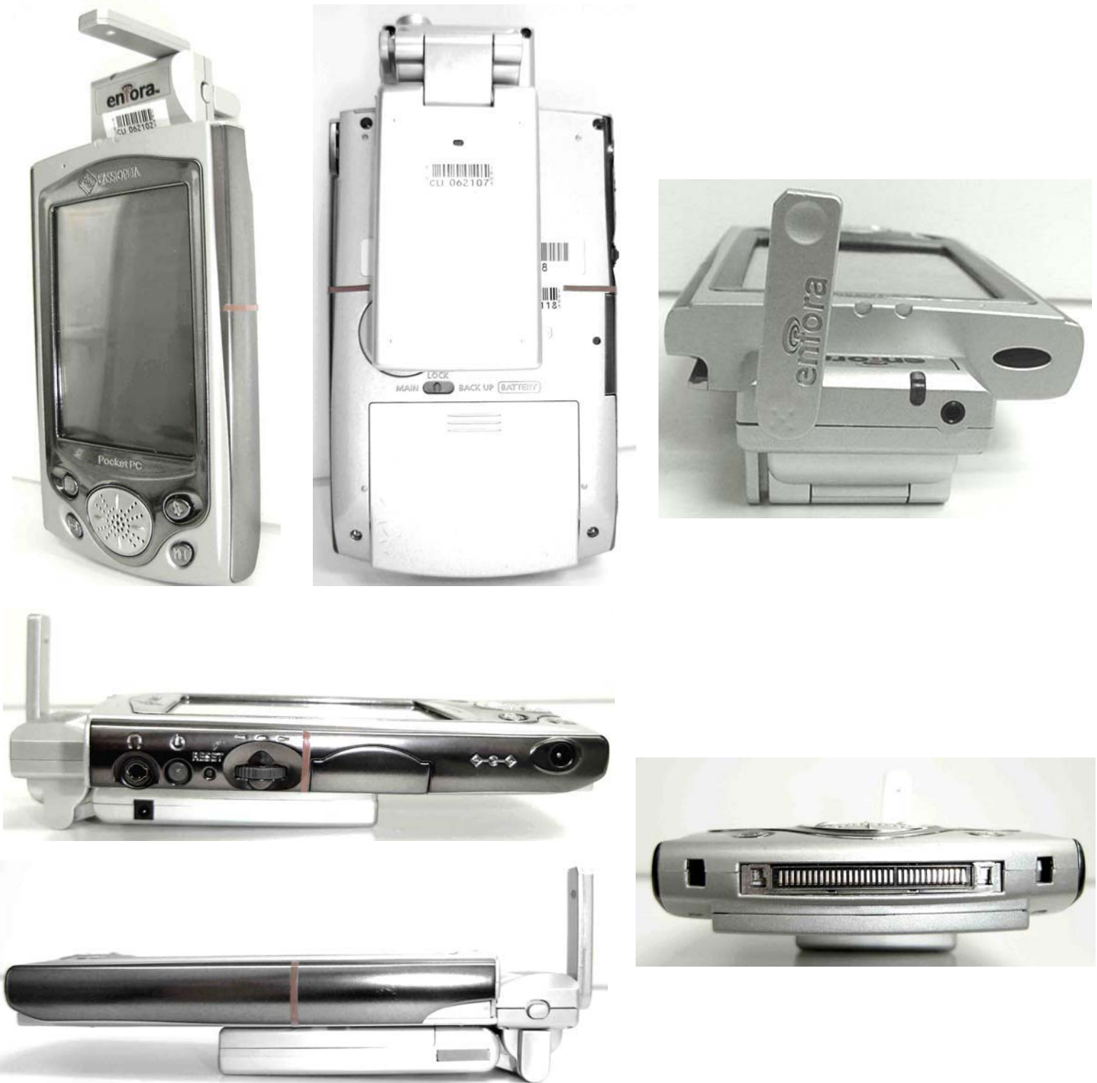
DUT in Compact Flash Slot of Casio E-200 PDA - with External DUT Battery
