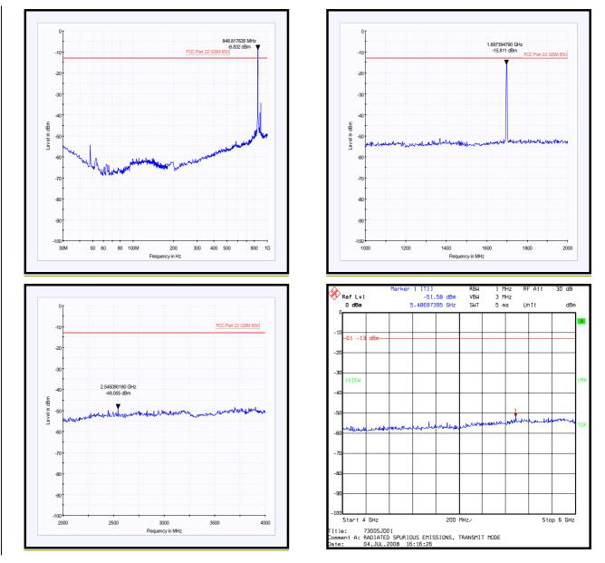
Note: These plots are pre-scans and for indication purposes only. For final measurements, see accompanying tables. Note: The emission shown at 848.817 MHz is the fundamental transmit frequency.
