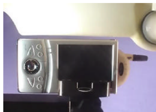
Body SAR Test Setup - Antenna Side of EUT (0.5 cm Separation Distance from PDA)
