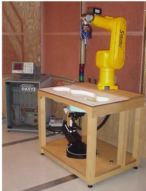
Figure 5. DASY3 SAR Measurement System
