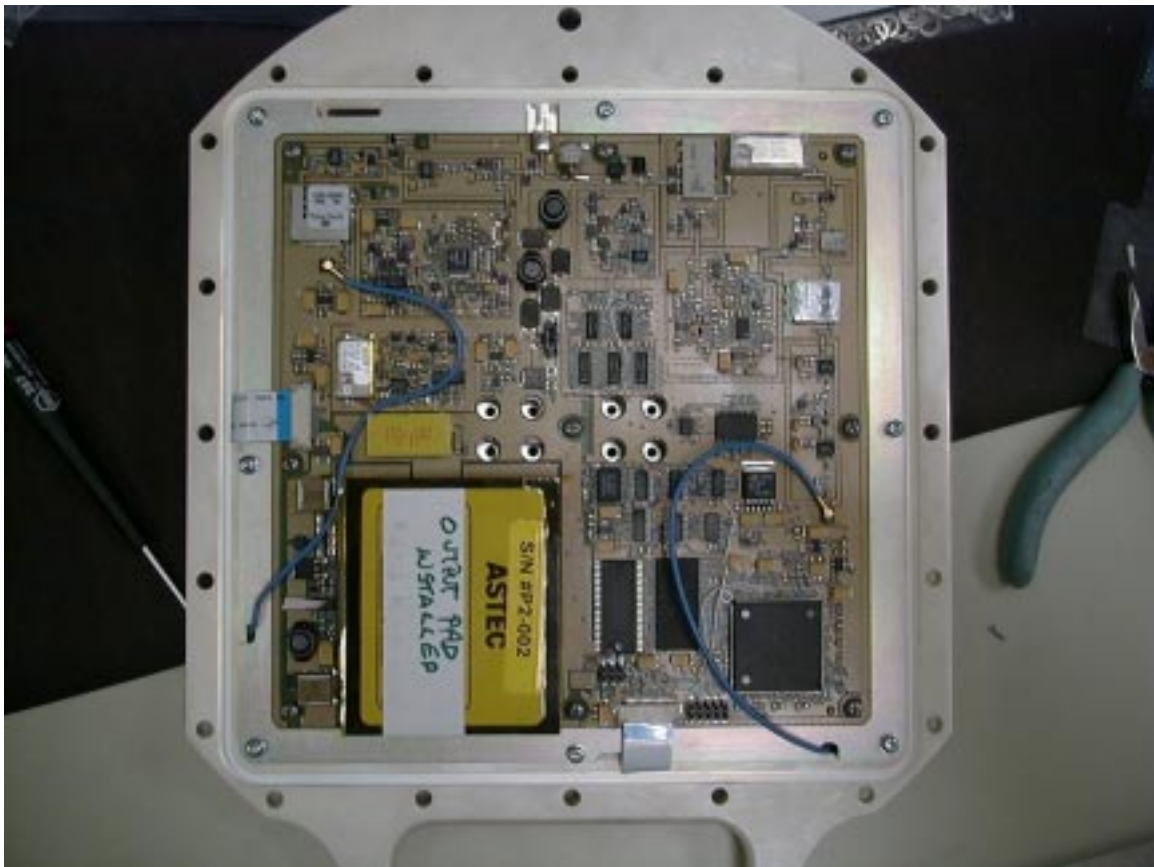
Figure 9.0-1 The Translator Assembly components are soldered/attached to a multi-layer printed circuit board that is installed into the chassis on top of the Millimeter Wave and Micro-Wave covers.
