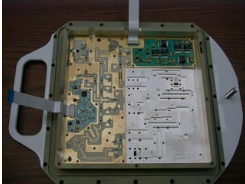
Figure 9.0-4 The Microwave assembly components are assembled onto a L-shaped 4-layer RF micro-strip circuit board to provide low-loss impedance matching interconnections for the signal flow paths. The exposed rectangular shaped portion of the chassis shows relief channels for RF paths and components for the Millimeter Wave Assembly not yet installed.
