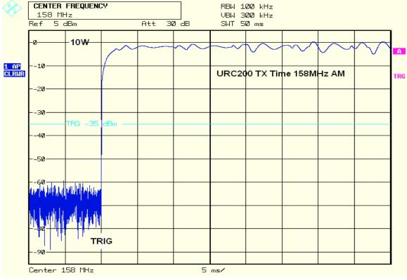
The results of testing the URC-200 rising RF envelope during the "Transmit Transient" condition is plotted below in FM 158 MHz.
