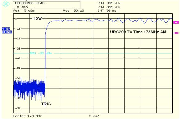
The results of testing the URC-200 rising RF envelope during the "Transmit Transient" condition is plotted below in FM 173 MHz.
