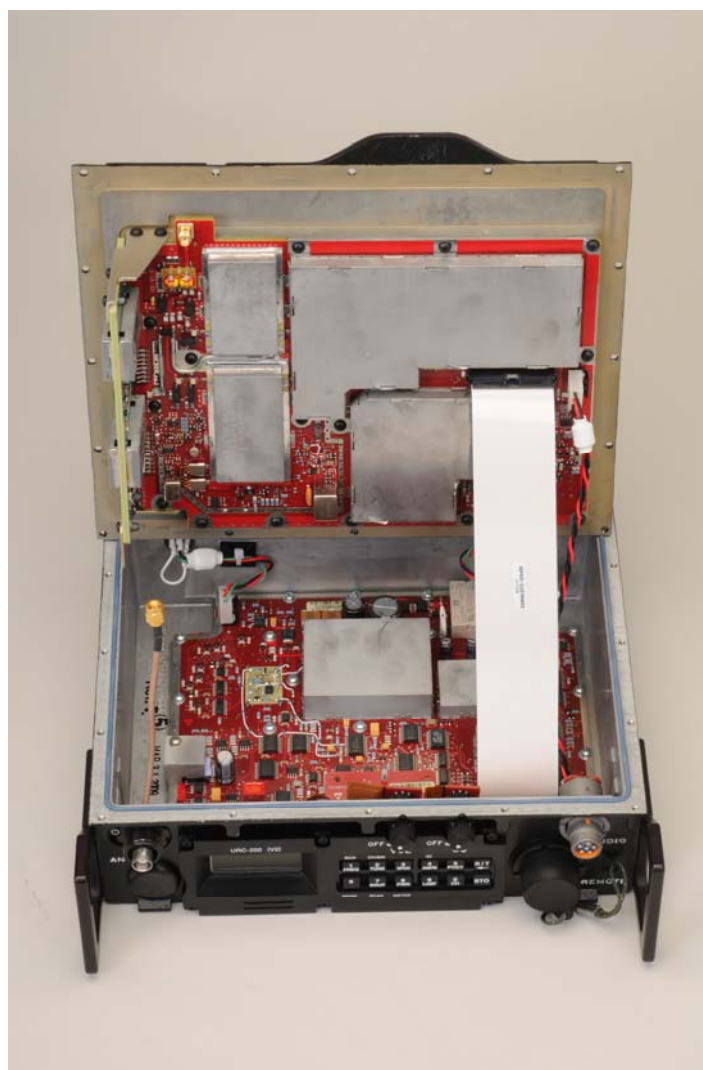
Figure 9.0-1 Cover opened illustrating PCB Layout
