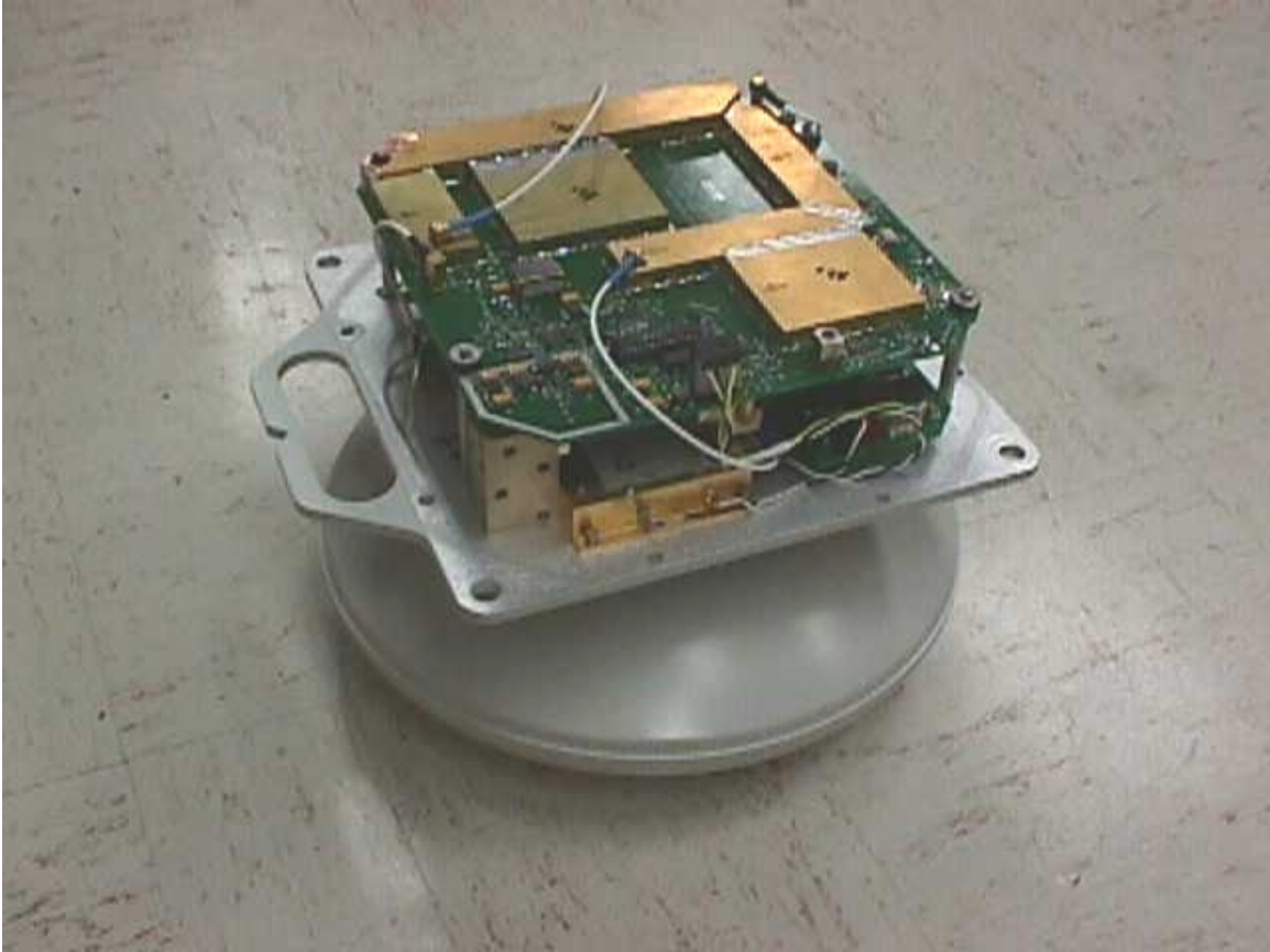
Figure 11.0-2 CPE Internal View
