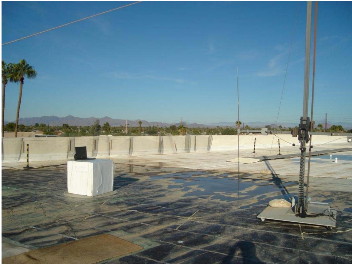
Radiated Emissions Test Configuration, OATS
