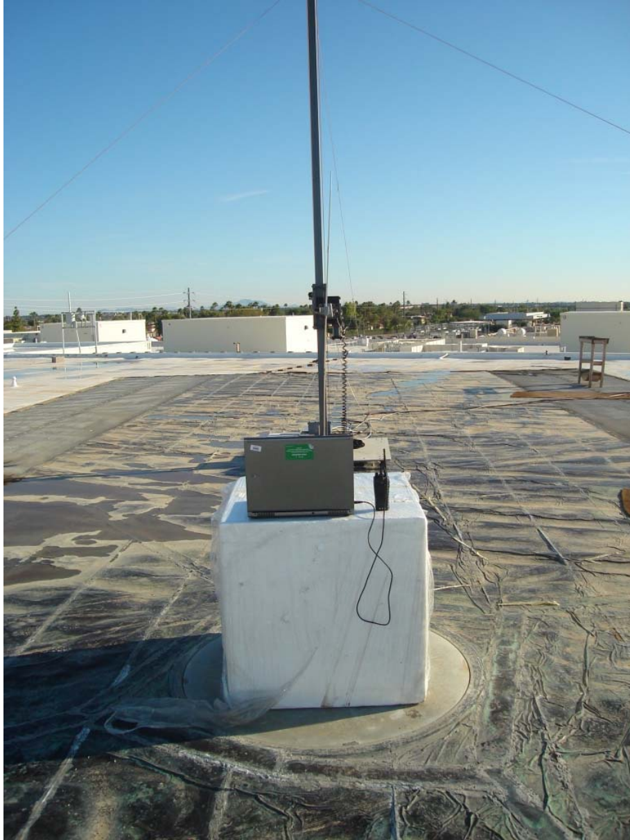
Radiated Emissions Test Configuration, OATS
