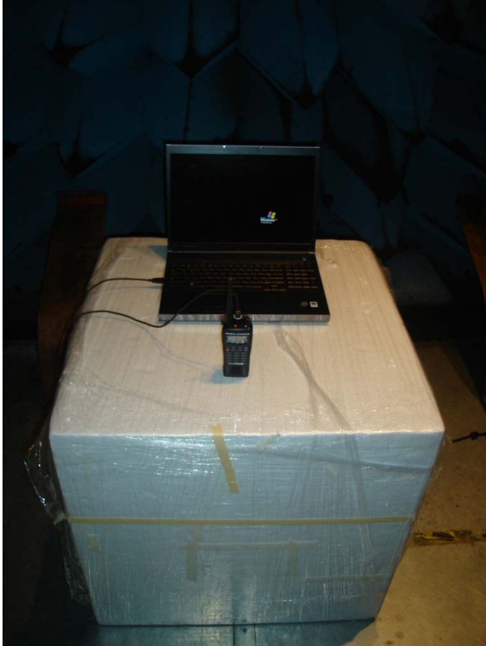
Radiated Emissions Test Configuration, Anechoic Chamber
